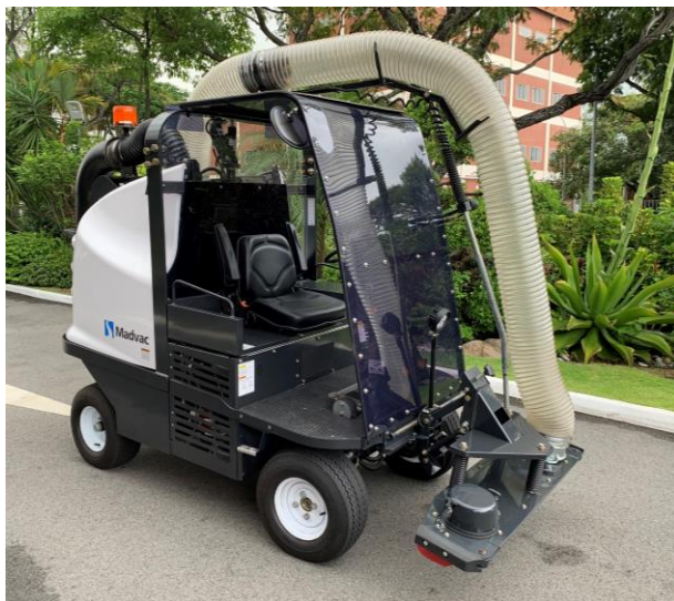
Tinted overhead shelter improves operator comfort & instrument protection
