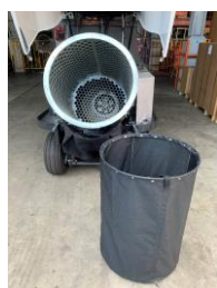
380L Hopper with debris basket
