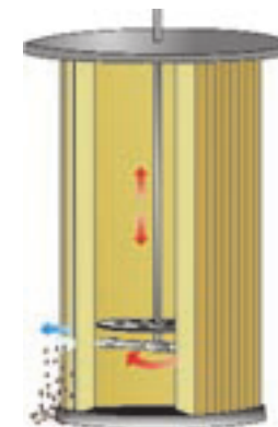
Manual cleaning with rotating jet of compressed air
