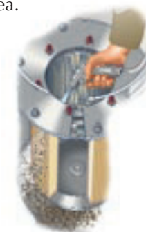
Cleaning with compressed air
